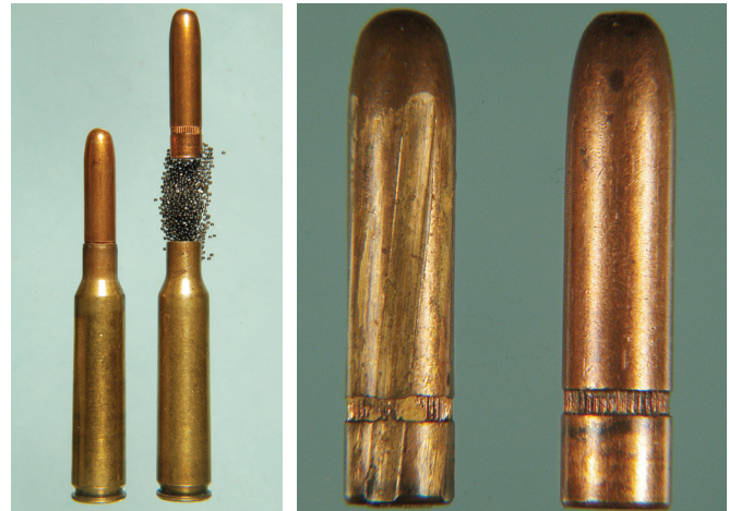
Figure 4: Western Cartridge Company 6.5mm Carcano cartridges (L), fired and unfired 160gr. WCC 6.5mm Carcano bullets (R)
