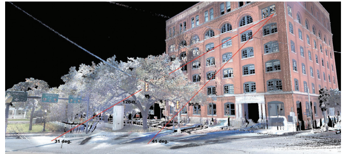
Figure 2: Leica® 3D laser scan with Elm Street intercept angles
