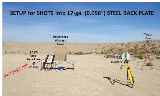
Figure 10: Velocity loss and deflection tests for traffic signal backplates
