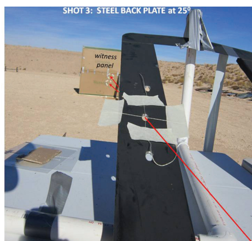
Figure 11: Velocity loss and deflection tests for traffic signal backplates
